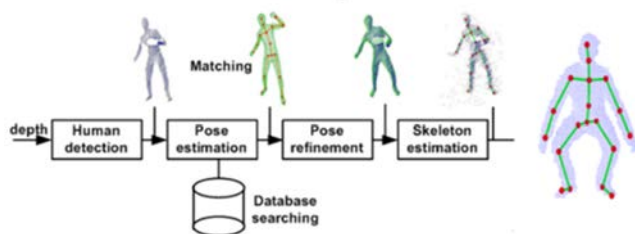
Fig. 4. Stages figure recognition by Kinect sensor [24]
